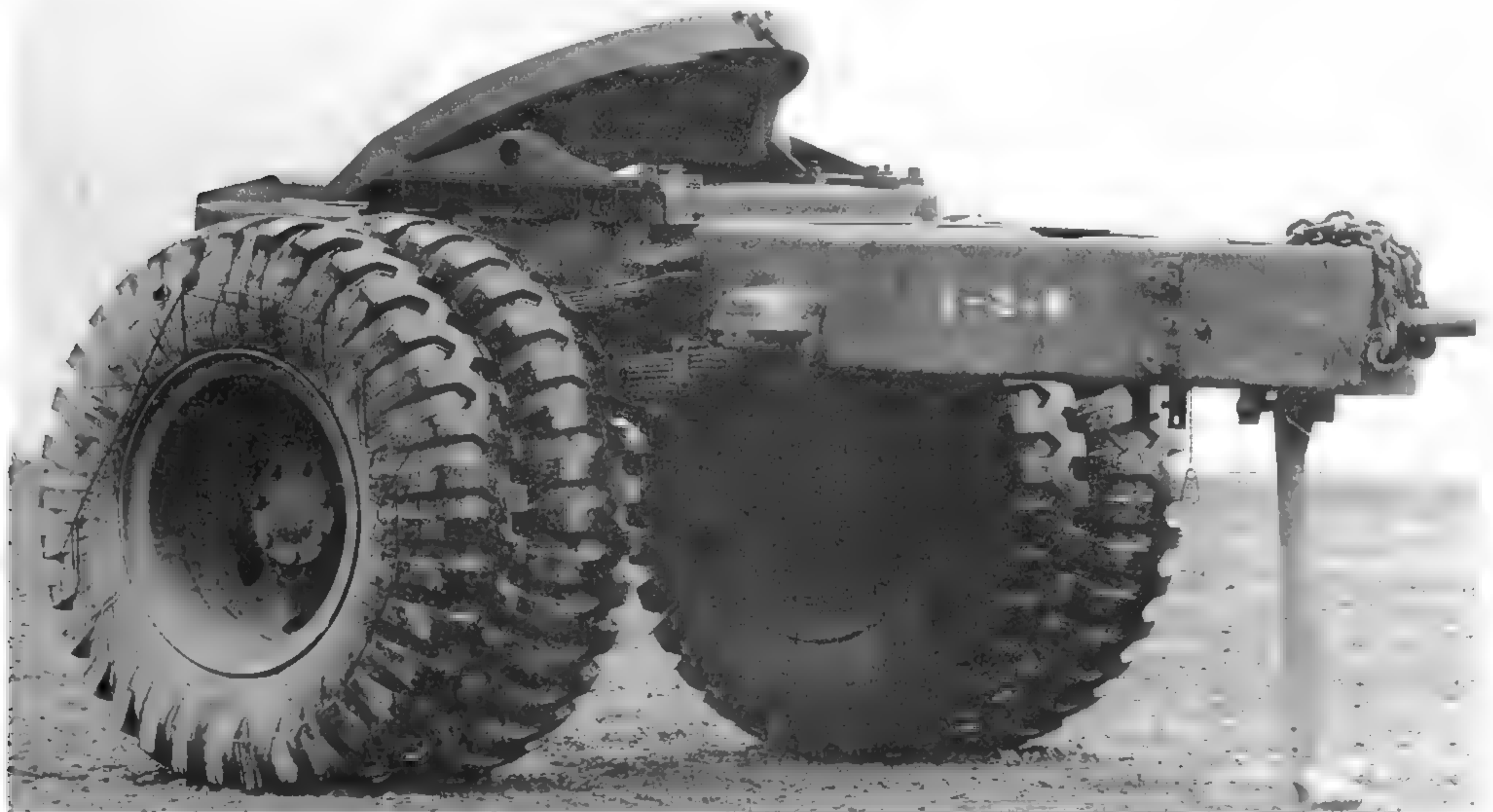
The M365 was the Army's heavy-duty converter dolly during WWII. Notice the overload springs mounted above the normal springs on this example built by Springfield Auto Works. (U.S. Army photo)
